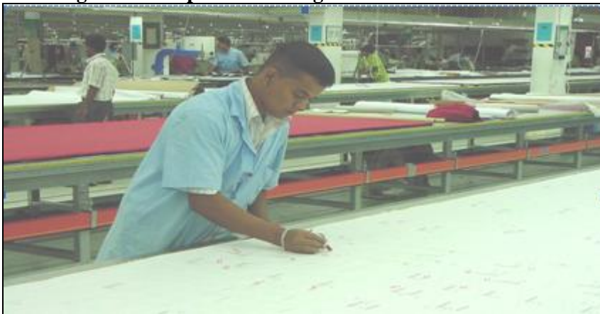
Checking of marker prior to cutting
